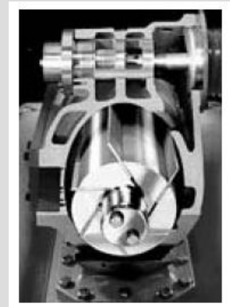
Figure 3.8 Cutaway view of a rotary vane compressor
