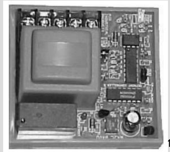
Figure 3.27 A defrost controller with timer
