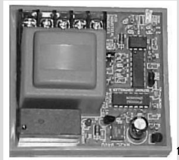
Figure 3.27 A defrost controller with timer
