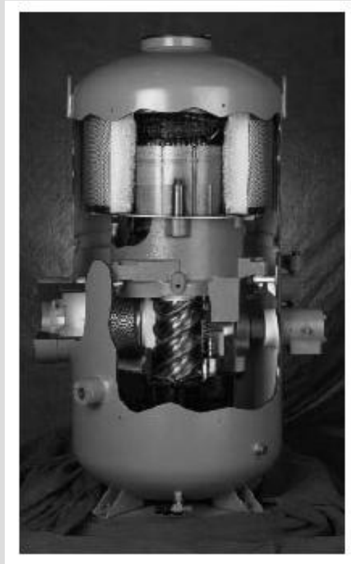
Figure 3.11 Internal view of a hermetic rotary screw compressor
