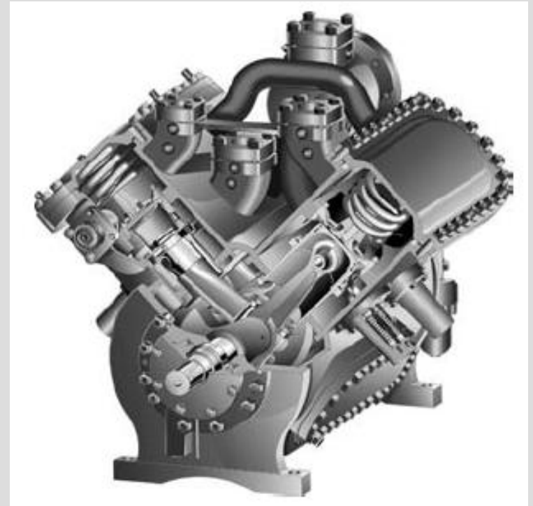
Figure 3.7 An internal view of V-type 6-cylinder reciprocating compressor
