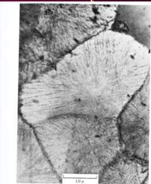
Fig. 5.76 (b) Identical composition heated rapidly to 875°C and held for 25 min. (from Fig. 5.76(a)).
