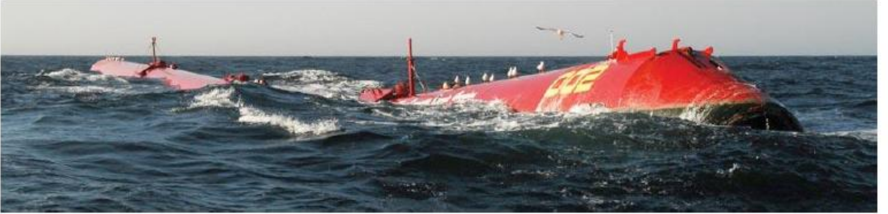
FIGURE 6-26 A wave power system using Pelamis technology ( www.pelamiswave.com )
